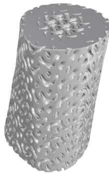
Figure 59. Femur bone section with graded density lattice structure (Gyroid) driven by CT-Scan data.
