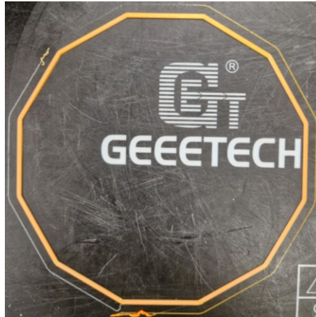
Figure 86. Deposition test (dodecagon shape) ASA-TPU additively manufactured.
