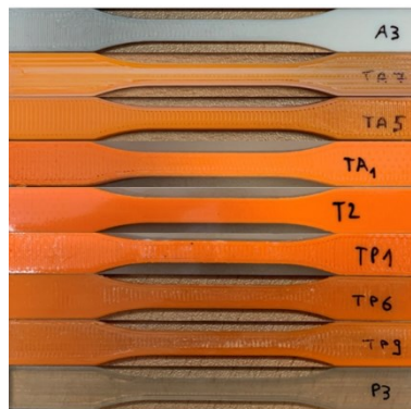
Figure 96. Tensile test samples, from top to bottom: 100% ASA, 75% ASA - 25% TPU, 50% ASA - 50% TPU, 25% ASA - 75% TPU, 100% TPU; 25% PLA - 75% TPU, 50% PLA - 50% TPU, 75% PLA - 25% TPU, 100% PLA.
