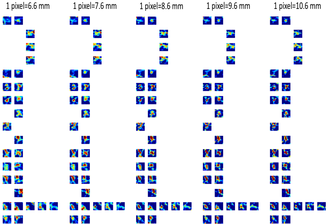
Figure 4.23: 2D reconstructions of the beam emissivity with 28 regions of different dimensions, subdivided in 11x11 pixels each.
