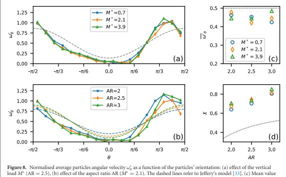
of the  $\omega'_{\theta}$  function and (d) parameter  $\chi$  as a function of the particles' aspect ratio (same legend as figure 8(c)). The black-dotted line represents the values obtained from the Jeffery's model [33].
