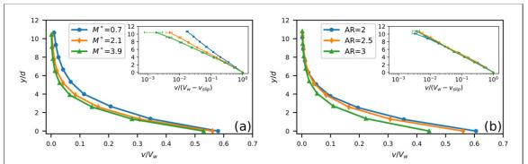
**Figure 3.** Time averaged translational velocity profiles: (a) effect of the vertical load  $M^*$  (AR = 2.5), (b) effect of the aspect ratio AR ( $M^* = 2.1$ ). Velocity is normalised by the wall velocity  $V_w$ . The error bars are smaller than the size of the data markers. The insets report the velocity profiles normalised by the  $V_w - v_{slip}$  in log-lin scale.
