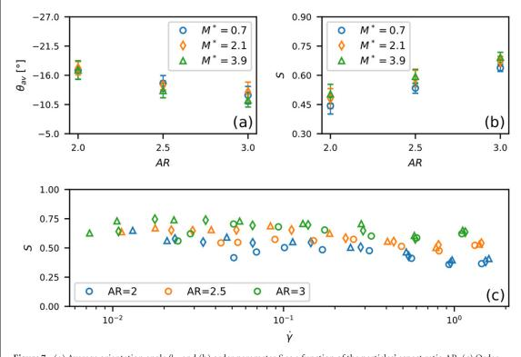
**Figure 7.** (a) Average orientation angle  $\theta_{av}$  and (b) order parameter *S* as a function of the particles' aspect ratio AR. (c) Order parameter *S* as a function of the shear rate  $\dot{\gamma}$ . The confinement level is indicated with different symbols:  $M^* = 0.7$  (o),  $M^* = 2.1$  ( $\Diamond$ ),  $M^* = 3.9$  ( $\triangle$ ).
