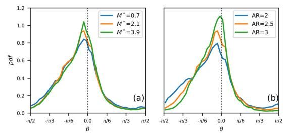
**Figure 6.** (a) Distribution of the particles' orientation  $\theta$ : (a) effect of the vertical load  $M^*$  (AR = 2.5) and (b) effect of the aspect ratio AR ( $M^* = 2.1$ ).
