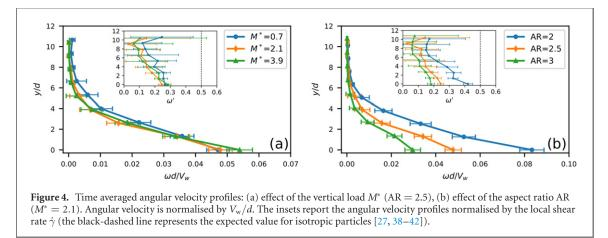
than 0.5, independently of the considered aspect ratio and of the flow region. This reveals that there is a geometric frustration of the particles' rotation due the shape anisotropy of the particles.
