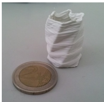
Figure 15 Ceramic vase 3D printed with composition H0 and heat treated at 1000°C for 1h.
