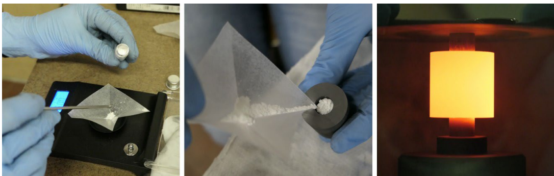
Figure 79. ^{nat}\text{ZnO} pellet preparation and graphite matrix inside the vacuum chamber during the process.
