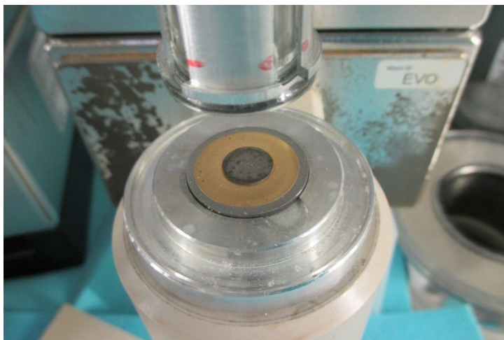
Figure 75. ^{nat}\text{Cr} target after the irradiation.
