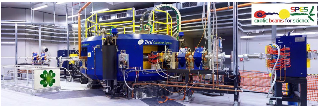
Figure 11. The new high-energy (35-70 MeV) and high-current (up to 750 \mu A) BCSI, model 70p proton-beam cyclotron installed at INFN-LNL (Legnaro, Padua, Italy).
