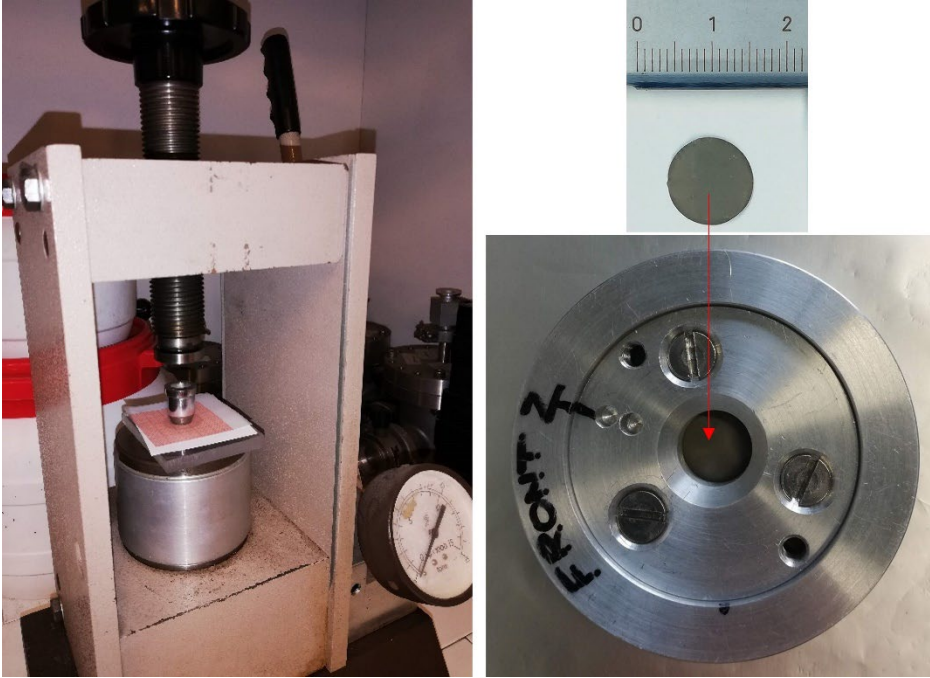
Figure 53. Left: hydraulic press used to cut the enriched Ti targets. Right top: picture of the cut target. Right bottom: assembled stacked foils target inside the sample-holder used for the irradiation at ARRONAX facility.
