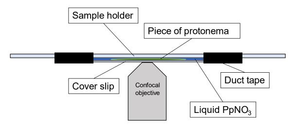
Supplementary Figure 4.9 | The setup used for sample mounting.
