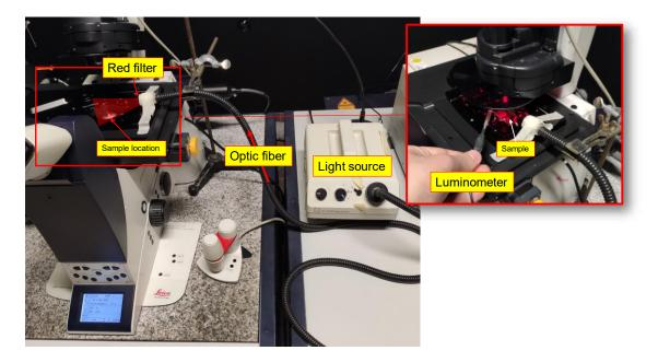
Supplementary Figure 4.10 | The setup used for monitoring of cytosolic ATP levels during darkto-light transitions. The image at right shows a detail of a illuminated sample, with light intensity being monitored with the probe of a luminometer.
