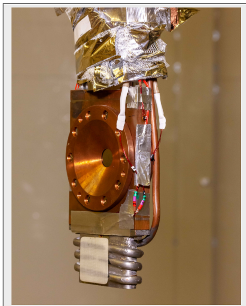
Figure 4.16: Picture of the copper target cell. The aperture cone faces backward angles towards the beam. A thermal shield is placed around the structure to offer insulation from the radiated heat from the surroundings. Figure adapted from reference [7].
