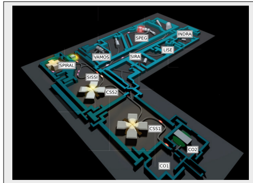
Figure 4.2: The facility for the production of post-accelerated radioactive beams in GANIL. Adapted from reference [17].
