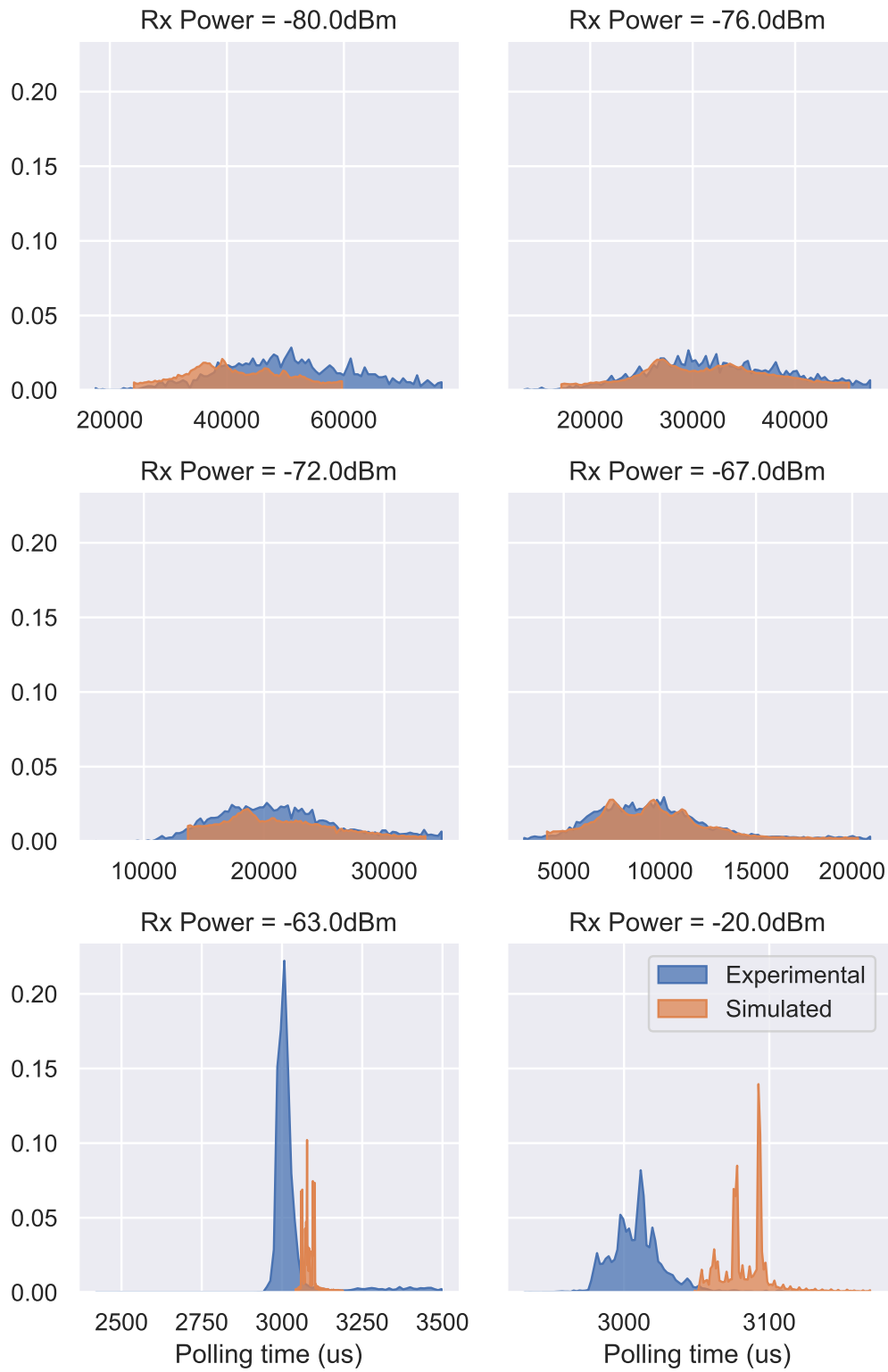
Figure 4.14: Comparison of the probability density function of the polling time in the experimental and simulated setup
