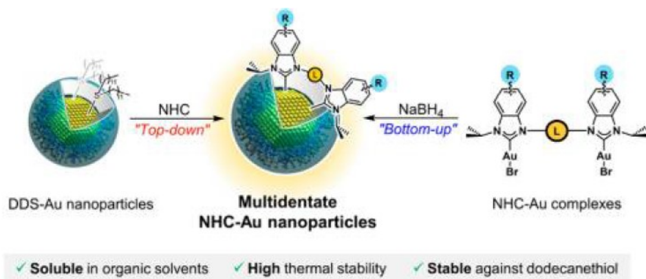
Figure 74: AuNPs protected with bidentate NHC synthesized via "top-down" and "bottom-up" approaches 31
