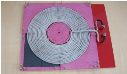
Fig. 4. Experimental coil without upper enclosure plate.
