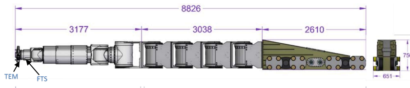
Figure 4.12: HYRMAN Concept Design overall dimensions in its full-length configuration [133]
