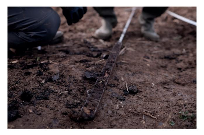
**Figure 5.1.** Wetlands are particularly suited for hand auger observations. This low-cost technique permits us to reconstruct the vertical stacking of peat (pictured) and other wetland sediments, such as organic or carbonatic muds or clastic sediments. This picture was taken by Sabrina Bianco during the University of Padova campaign in the Fimon lake area (Berici hills, Veneto, northeast Italy) in 2019. Image: Sabrina Bianco.
