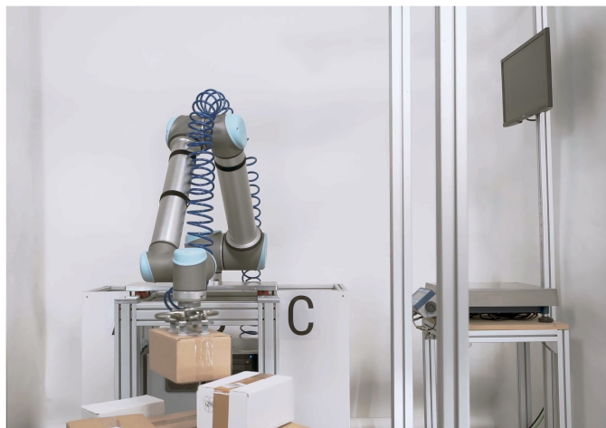
Fig. 1. Example of workcell. A UR10 pick up randomly placed boxes and places them on a delivery tracking system.
