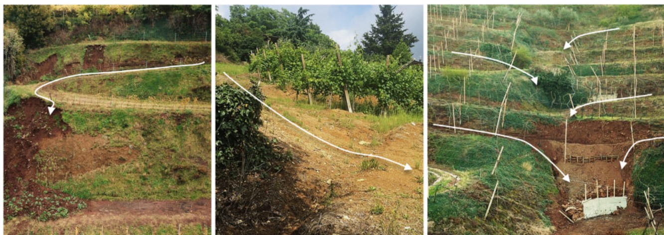
FIGURE 5 Field evidence of common erosive processes directly related to geomorphologic elements of vineyards, highlighted by white arrows. On the left, sheet erosion and a series of shallow landslides were caused by runoff from zigzagging roads. In the centre, an eroded steep lateral access road to a terraced vineyard. On the right, a series of terrace collapses downstream of a hillslope with concave sinuosity. [Photographs by T.A. Vogel (left, right) and E. Quarella (centre)] [Colour figure can be viewed at wileyonlinelibrary.com ]
