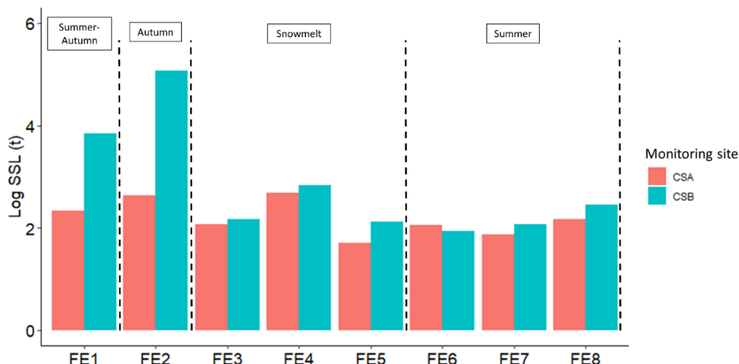
Figure 4.5. The logarithmic value of suspended sediment load registered at the upstream (CSA) and downstream (CSB) sites for each of the eight events recorded during the monitoring period. The FE1 occurred between the 29 th August and 9 th September 2020, the FE2 between 2 nd and 10 th October 2020, the FE3 between the 1 st and 6 th May 2021, the FE4 between 8 th and 15 th May 2021, the FE5 between 23 rd of May and 16 th June 2021, the FE6 between 8 th and 13 th July 2021, the FE7 between the 13 th and 19 th July 2021 while the FE8 between the 4 th and 9 th August 2021.
