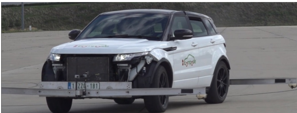
Figure 1.: The iCOMPOSE electric vehicle demonstrator with the Corrsys Datron sensor installed on the front end (Lommel proving ground, Belgium).
