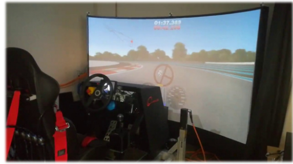
Fig. 1. Compact dynamic driving simulator is composed of a cockpit, an active belt and active seat system, four legs for tilting and vertical motion, a high-resolution cylindrical screen, and a high-fidelity vehicle simulation software (VI-CRT).
