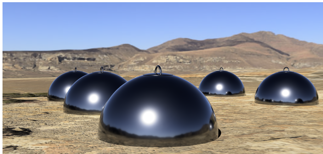
Figure 8. Illustrative rendering of several hemispherical detector units deployed on a high-altitude plateau, representing a possible configuration of the outer array. The compact, low-profile aluminium shells are designed for simple placement on prepared foundations, with the instrumented bladders inserted from the top hatch after installation and connected to power and readout services via standardised external interfaces.
