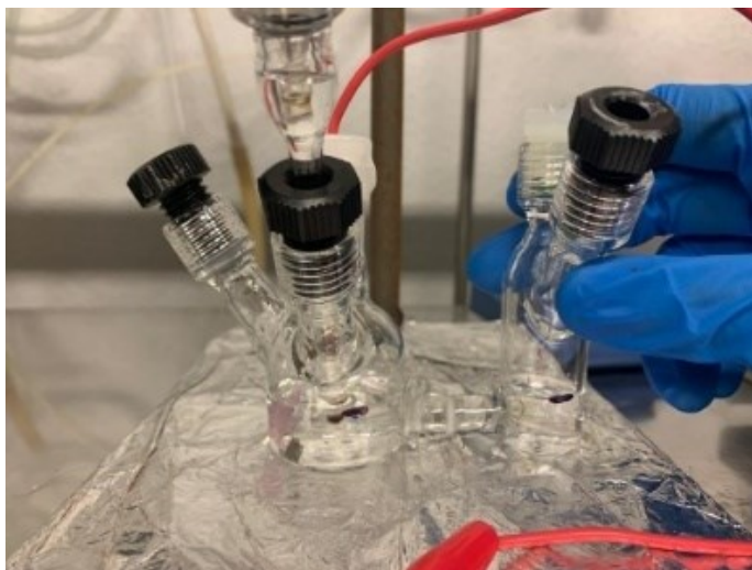
Figure 139. Two-compartment photoelectrochemical cell used to study QNC-based photoanodes in gas-tight conditions.
