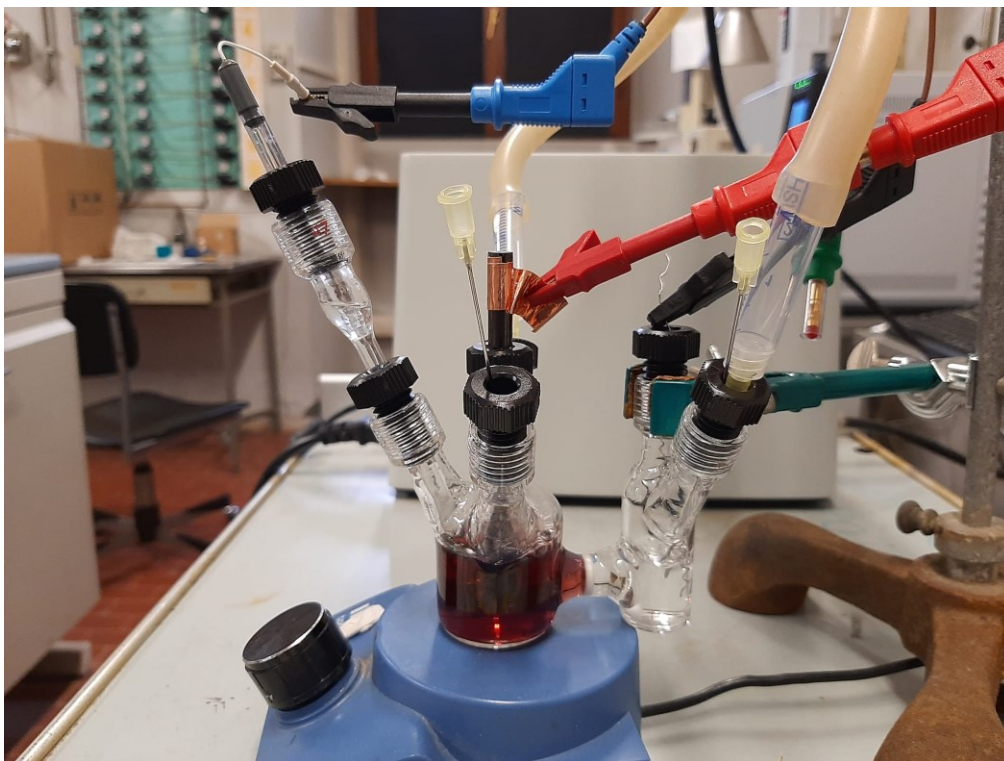
Figure 88. Gas-tight electrolysis cell used throughout the study. The working compartment, containing the coloured solution, and the auxiliary compartment, are shown being degassed. Electrodes and connections are assembled as described in the text. The salt bridge housing the RE is visible.
