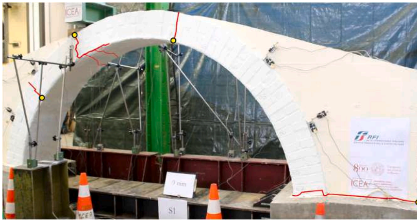
Fig. 10. Deformed shape of the strengthened arch at 9 mm imposed displacement.
