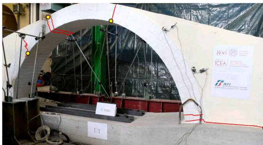
Fig. 7. Deformed shape of the unstrengthened arch at the load peak: activation of the principal mechanism (B1).
