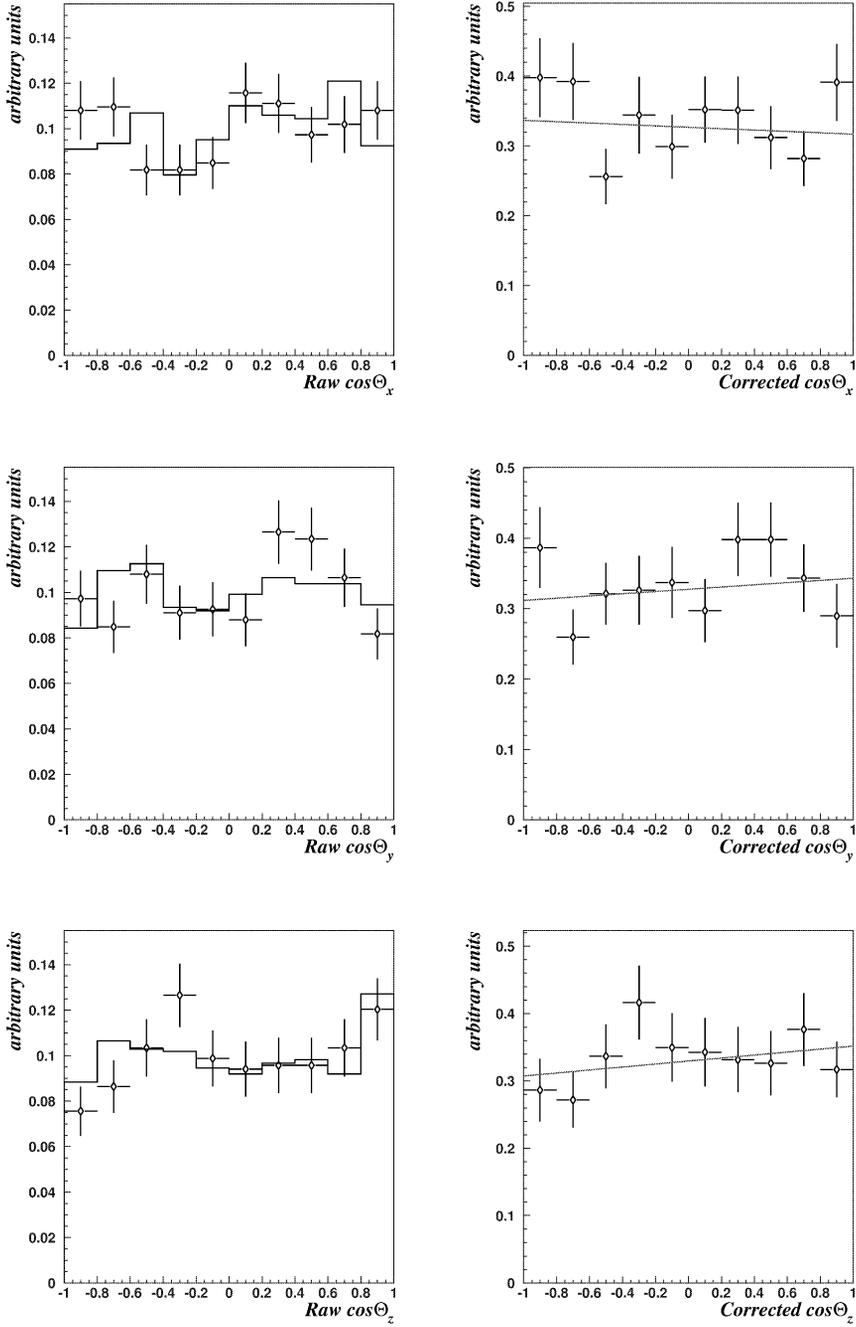
Fig. 4. Left: normalized angular distributions ( $\cos\theta_i$ ) for  $\bar{\Lambda}$  hyperons in reconstructed Monte Carlo events (histogram) and in data (points with error bars). Right: experimental angular distributions corrected for detector acceptance and selection effects; the polarization is given by the slope of the corresponding linear fit.
