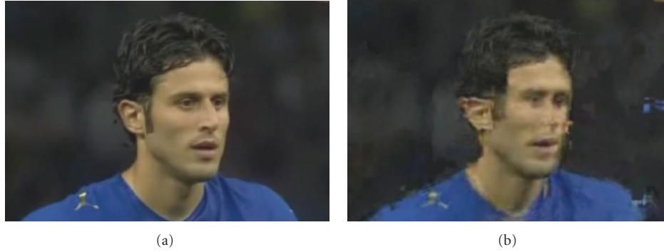
FIGURE 4: First scenario, multicast video streaming, SIR = 4 dB: (a) original frame, (b) corrupted frame.
