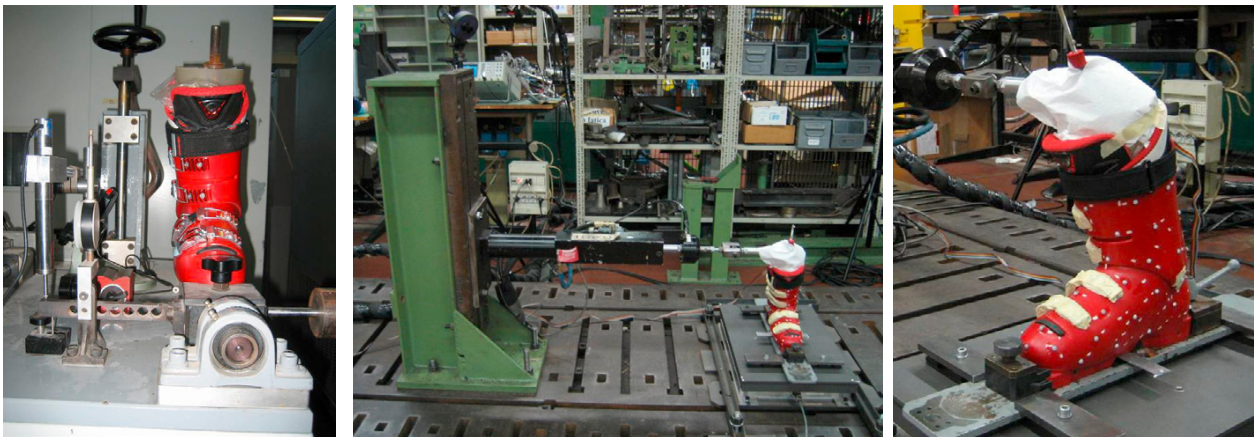
Fig.2. The Laboratory tests. (a) Torsional stiffness test setup; (b) Lateral stiffness tests setup. (c) Motion Capture setup for the collection of the boot displacement patterns during lateral bending.
