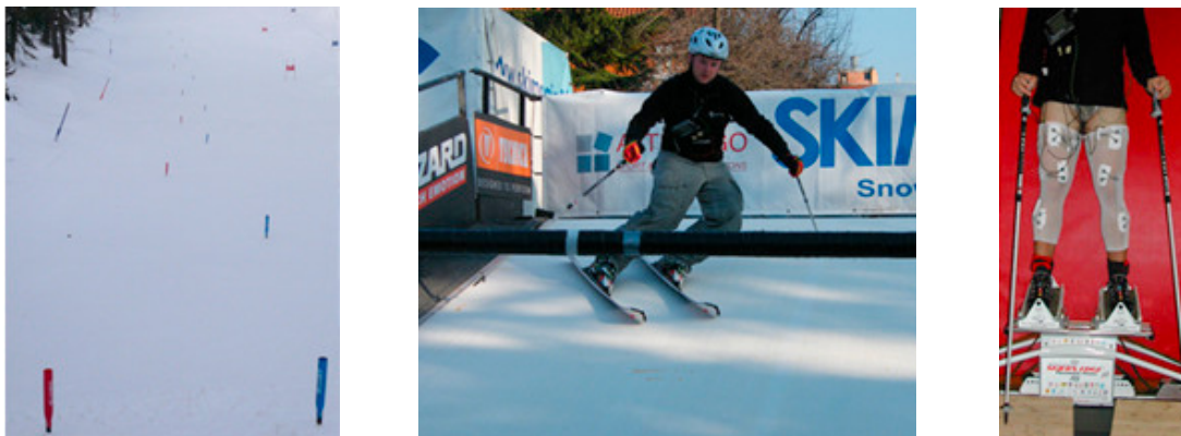
Fig.1. Set-up of the different sessions: (a) Natural slope; (b) Skimagic®; (c) Skier's Edge®
