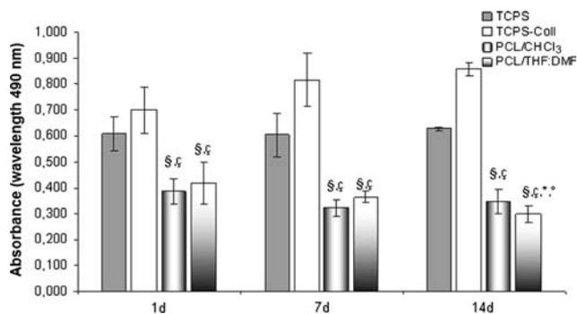
Fig. 3 HA viability evaluated with MTS assay for tissue culture plate scaffold (TCPS), collagen-coated TCPS, microbrous (PCL/CHCl<sub>3</sub>) and submicrobrous matrices (PCL/THF:DMF) ( $P < 0.05$  with respect to TCPS;  $P < 0.05$  with respect to collagen-coated TCPS; \*  $P < 0.05$  with respect to 1 day;  $P < 0.05$  with respect to 7 days)
