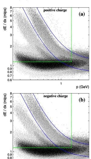
Fig. 2. The dE/dx distribution as a function of the track momentum for: (a) positive and (b) negative tracks. The dE/dx is normalised to a minimum ionising particle, defined as the average truncated mean of pion tracks in the momentum range 0.3 GeV. The solid lines indicate the (anti)proton bands used in this analysis, and the dotted line denotes the cuts <math>dE/dx > 1.15 mips and p < 1.5 GeV.
