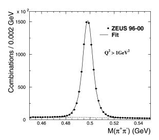
Fig. 1. The  $\pi^+\pi^-$  invariant-mass distribution for  $Q^2>1~{\rm GeV}^2$ . The solid line shows the fit result using a double Gaussian plus a linear background, while the dashed line shows the linear background.
