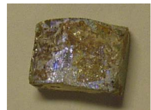
Figure 2. Tessera with pale gold leaf (Au 01): the lateral faces with deterioration patinae
