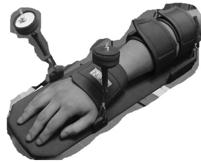
Fig. 3. NeReBot splint close-up. Patient's hand is supported by a hemispherical plastic component, while the forearm is fastened by three fabric strips. Front wire magnetic fasteners are also shown.
