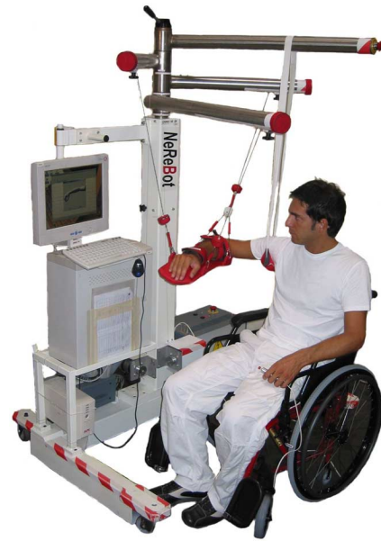
Fig. 1. NeReBot overall view. Patient's forearm is fastened onto a splint, which is moved by three directly-driven nylon wires. Graphical interface is used to keep the patient's attention focused on the exercise.
