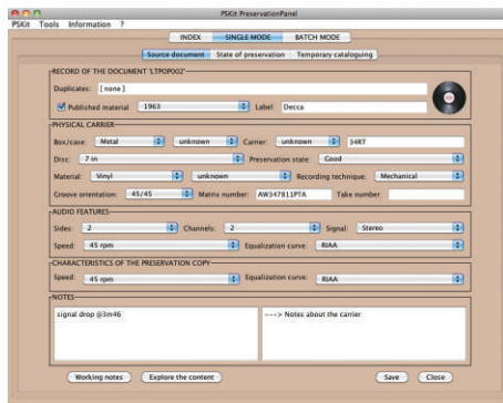
FIGURE 11: Panel for the description of single documents in PSKit PreservationPanel for the carrier type “phonographic disc.”
