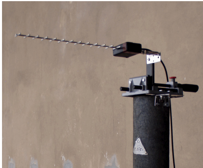
Figure A.2. One of the Yagi–Uda antennae of the interferometer mounted on the top of an isolated plastic pillar.
