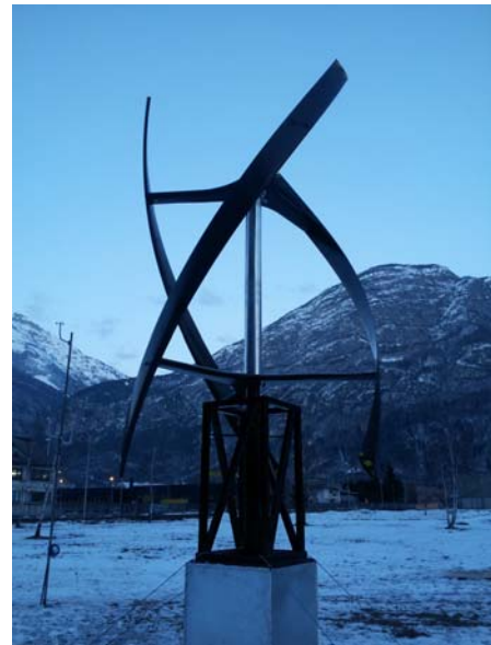
Fig. 1: VAWT tested in Longarone open wind facility, BL (Italy)
