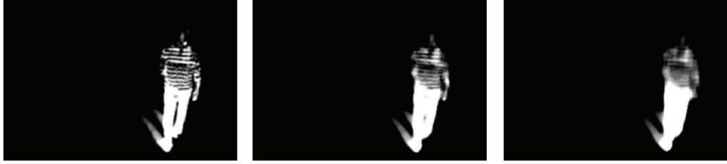
FIGURE 3: Example of confidence image after applying a median filter of size, respectively (from left to right): 3 \times 3 , 7 \times 7 , and 11 \times 11 .
