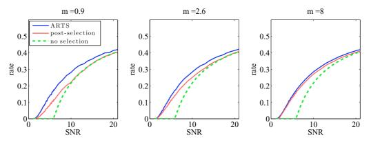
FIG. 6. (Color online) Comparison between the rates achievable by the ARTS, the postselection, and the standard QKD technique (no selection). We assumed that the channel QBER is 3% and the log-normal parameter is  $\sigma = 1$ , similar to the parameter we measured in the tested free-space channel. The parameter *m* represents the mean received bits per coherence time of the channel.
