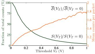
FIG. 3. (Color online) Mean counts per packet  $\overline{S}(V_T)$  (normalized to the mean counts obtained without thresholding) and fraction of total count  $S(V_T)/S(V_T = 0)$  in function of the probe threshold.
