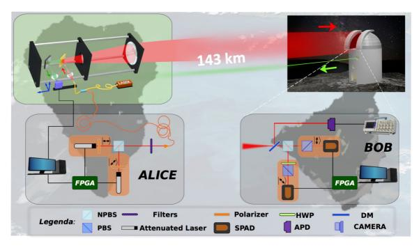
FIG. 1. (Color online) Experimental setup: Alice is located at JKT observatory in La Palma. Qubits are prepared using a field-programmable gate array (FPGA) controller, linear optical components, and attenuated lasers. Alice telescope is also configured to acquire the beacon beam sent by Bob, located at the Optical Ground Station in Tenerife, and used for tracking the transmitter in order to stabilize the pointing.
