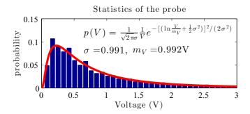
FIG. 4. (Color online) Experimental occurrences of probe intensities (measured by photodiode voltages) and log-normal fit.
