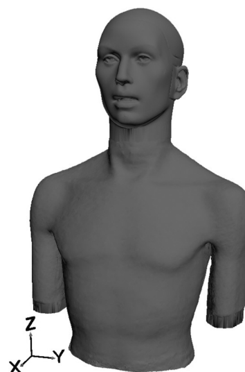
FIG. 1. 3D view of the used KEMAR mesh and the coordinate system.
