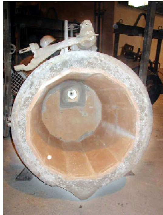
Fig. 10 Example of new lining materials with low density and low conductivity for ladles (courtesy of Foseco)
