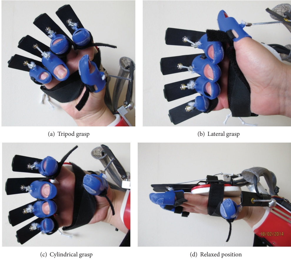
FIGURE 2: Selected gestures to be recognized performed wearing the SCRIPT device.
