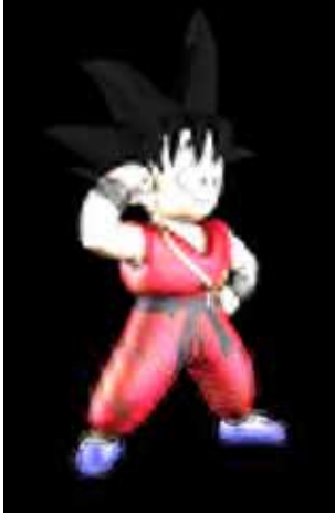
FIGURE 12: View of the Goku model corrupted by a loss in the first part of the texture codestream.
