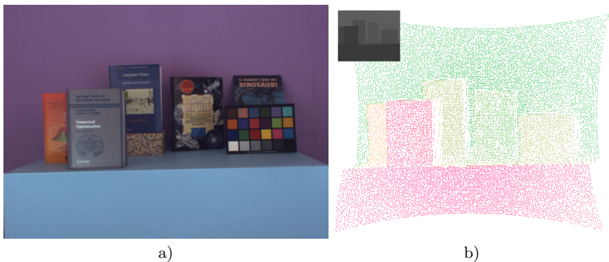
Fig. 1. Example of sparse disparity measurements: a) cropped color image framing the acquired scene; b) disparity data acquired by the ToF camera reprojected on the lattice associated to the left camera (the depth map acquired by the ToF camera is shown in the upper left corner at its original size).
