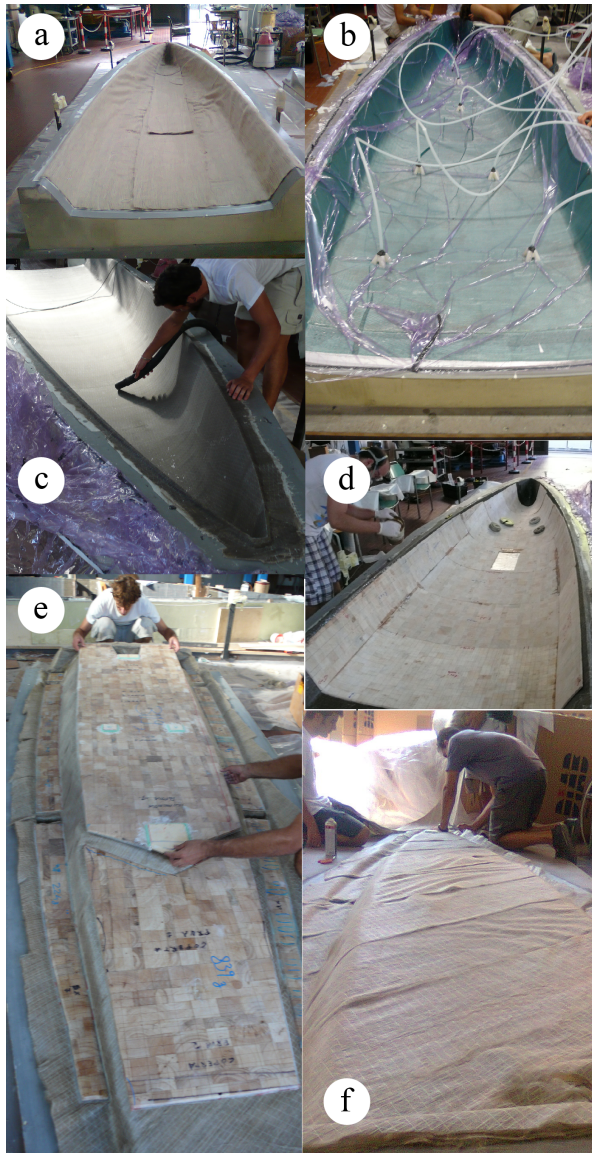
Figure 7: Some phases of the multi-step technique applied to realize the boat: a) Positioning of the flax fibers on the hull mould for the external skin; b) Infusion of the external skin; c) Preparation of the external skin before the vacuum bagging of the core; d) Handing-lay up of the core prior the vacuum bagging; e) - f) Preparation of the deck layers for the single infusion.
