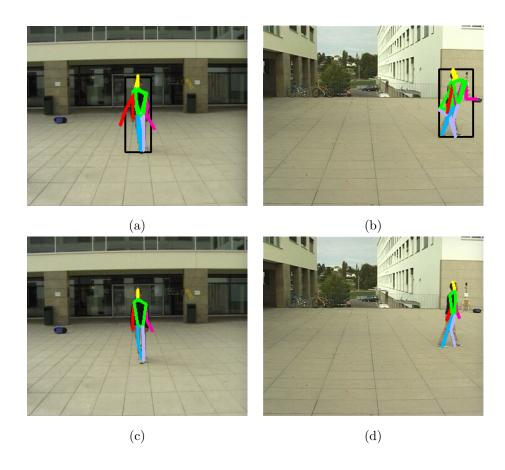
Figure 4: Two views showing the clustered skeletons (a-b) and the reprojections of the 3D triangulated points (c-d). It is possible to see that the processing in 3D world coordinates rejects the outliers that cause the wrong estimations of the arms.
