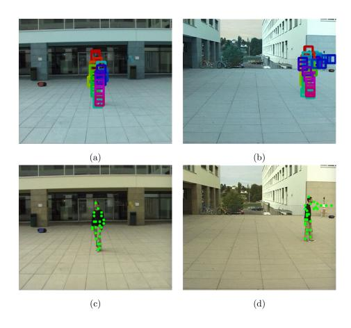
Figure 1: Sample of the output of the Part Based Detector on two images taken from two cameras with overlapping fields of view (a-b) and the corresponding keypoints evaluated by the system.
