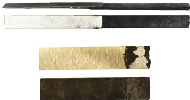
Figure 5. Shear strength specimen and fracture area after the test
