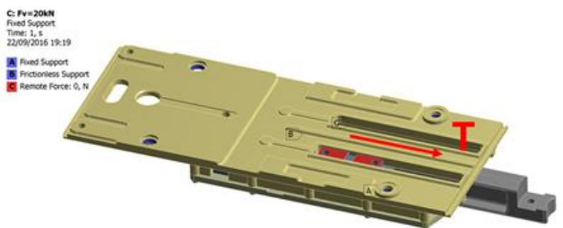
Figure 8. Boundary conditions for the half model comprising the detection rod.
