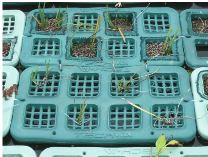
Figure 4. Particular of two TECH-IA® elements in which the plants were set with ( above ) or without ( below ) the substrate of expanded clay.
