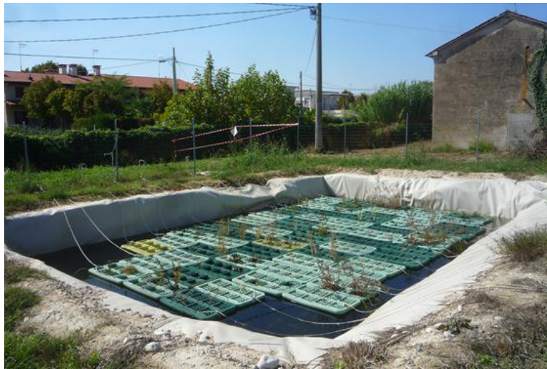
Figure 3. The bioretention pond at the end of the first growing season of the experiment.
