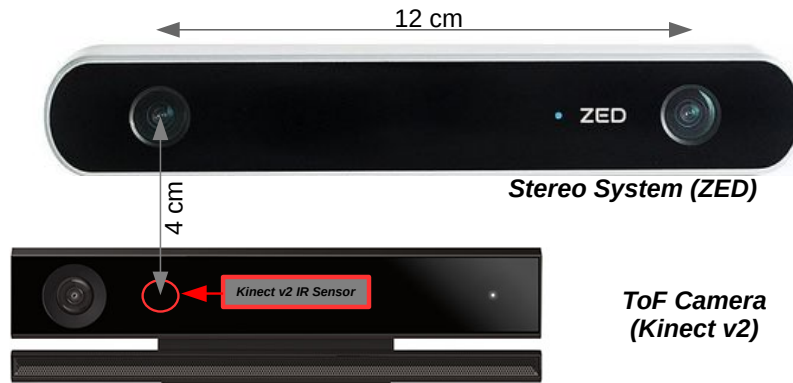
Figure 4: Representation of the real Stereo-ToF acquisition system. The Figure shows the relative position of the ZED camera and of the Kinect v2.
