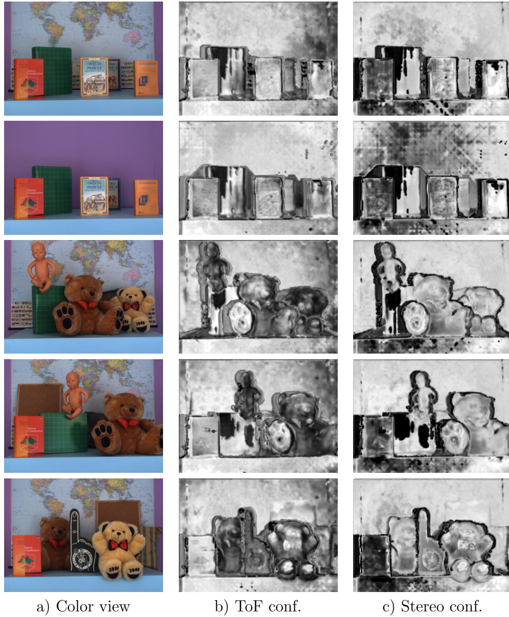
Figure 11: Confidence information computed by the proposed deep learning architecture for the scenes in the LTTM dataset: a) Color view; b) Estimated ToF confidence; c) Estimated stereo confidence. Brighter areas correspond to higher confidence values, while darker pixels to low confidence ones.
