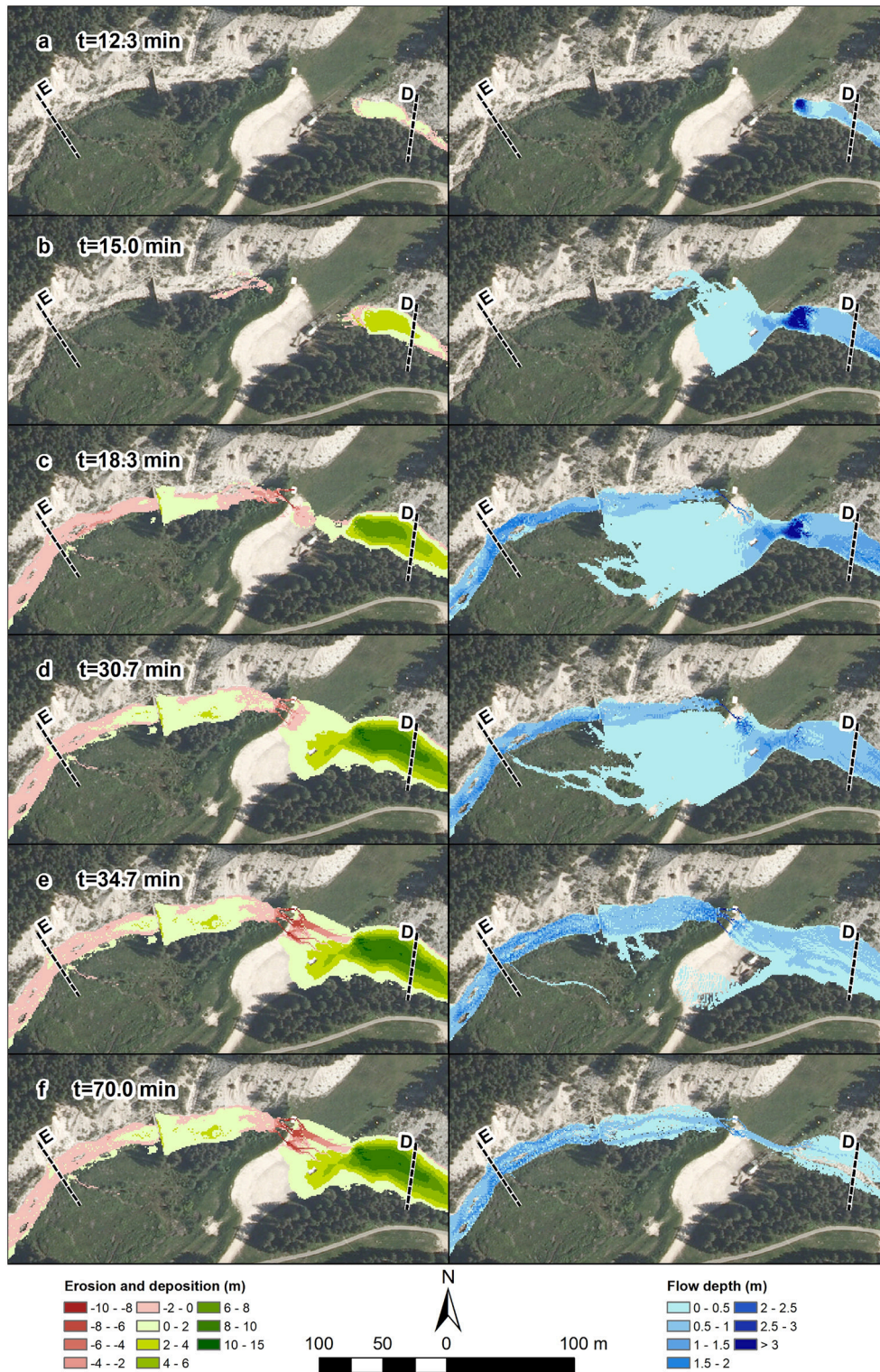
FIGURE 12 | The deposition and erosion depths (Left) and flow depths (Right) maps at different times [(a) t = 12.3 min, (b) t = 15.0 min, (c) t = 18.3 min, (d) t = 30.7 min, (e) t = 34.7 min, (f) t = 70.0 min] from the beginning of the simulation of the area close to the culvert and parking.
