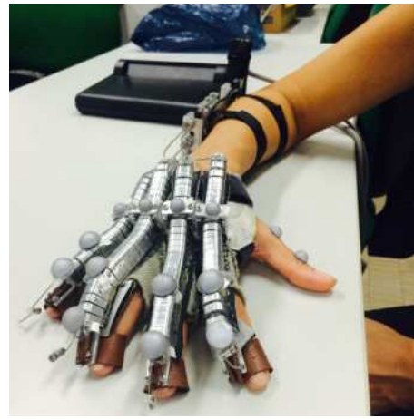
Fig.9 - FEX device tested for being possible to wear even during very complex tasks like handshake and to be able to force open semi-closed fingers (left), FEX device with markers glued onto (right).
