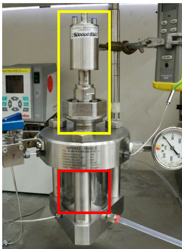
Picture of the HPU+scCO 2 drying reactor. High pressure reactor with the sonotrode; the drying chamber is highlighted in red, while the HPU sonotrode in yellow.
