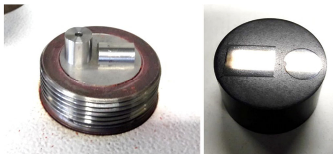
Fig. 5 - Sample preparation for micrographies, in particular the resin embedded sample (longitudinal and cross sections) is depicted on the right
