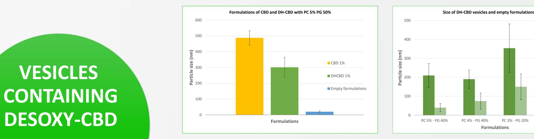
Vesicles containing DH-CBD or CBD were prepared by simple mixing method with a mechanical stirrer<sup>4</sup>. The effect of variable concentrations of propylene glycol (PG) ranging from 20 to 50% in systems containing DH-CBD were observed. Particle size was measured by DLS and optimal results were generally given by formulations with 40% PG, in which vesicle size was maintained at around 200 nm.
