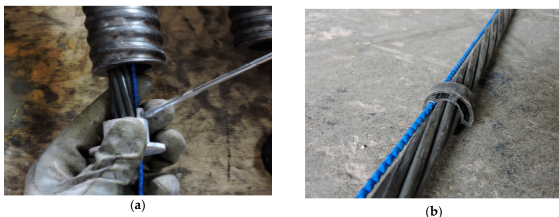
Figure 3. Plastic hooks for coupling the DFOS (distributed fibre optic sensors) to the tendon in a composite bar: (a) element for extremity; (b) internal element.
